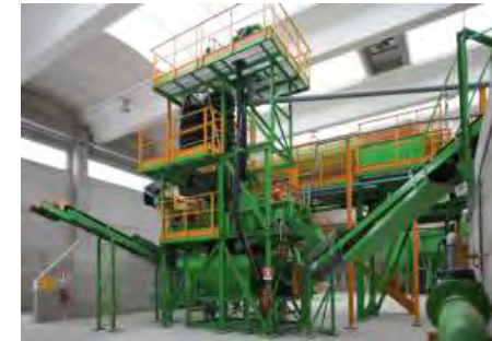
Street sweepings recovery plant Milano Capacity: 30 kt/a
