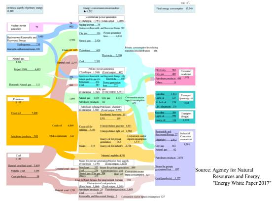
Figure 2-1 Domestic Energy Balance and Flow (Overview) (FY 2015)
