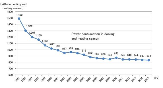
Figure 2-27 Progress of energy saving for air conditioners
